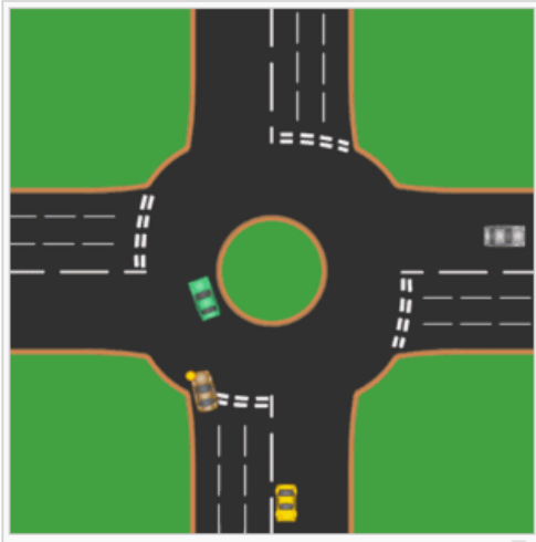
Figure 3. A roundabout for traffic flowing on the left side
