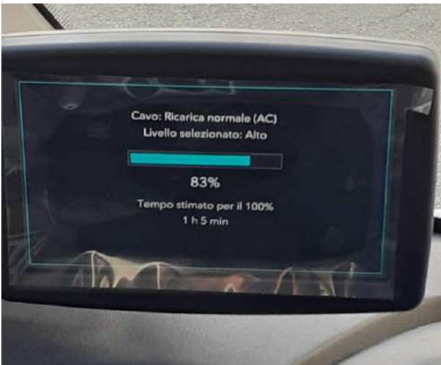
Image 16. Control monitor representing the actual values for the completion of the charging process.
