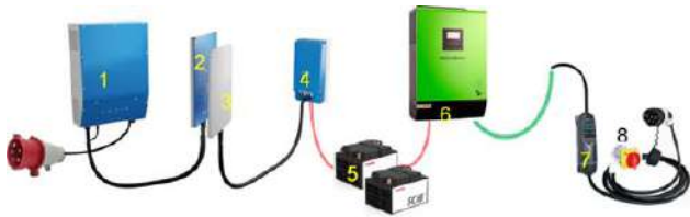
Image 6. Architecture of the wireless charging system. The ground section is made up of elements 1 and 2, while the section on board the vehicle is made up of equipment 3, 4, 5, 6, 7 and 8.
