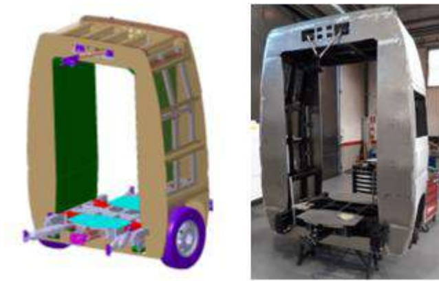
Image 20. Bodywork of the flexible joint.
