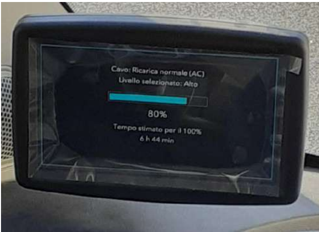
Image 15. Control monitor representing the estimation for the completion of the charging process.
