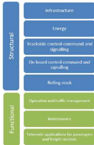
Figure 8. Rail Subsystems according Directive EU 2016/797 Annex II
