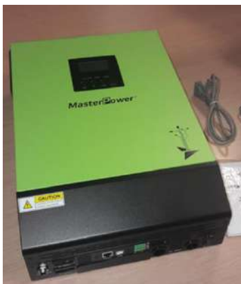
Image 12. Photograph of the DC-AC inverter.
