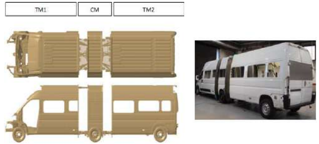
Image 22. Coupling scheme between all modules [TM1 + CM + TM2] (left) and their photographic rendering (right).
