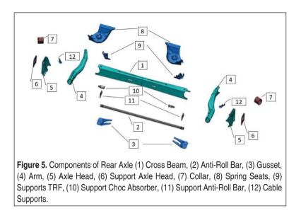
All these components are being produced by stamping, machining, roll forming, forging, etc. The production method has been decided at the beginning of the project for each component based on the vehicle requirements along with the material grade and the thickness.
