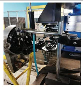
Figure 7. Durability Performance Test Bench With Automatic Control For Rear Axles
