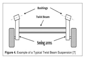
The axle that will be worked on for the scope of this paper is a H shaped twist axle. There are several components that need to be joined properly to be able to provide the necessary performance for the duration of the vehicle life. The parts of the axle are joined via GMAW.
