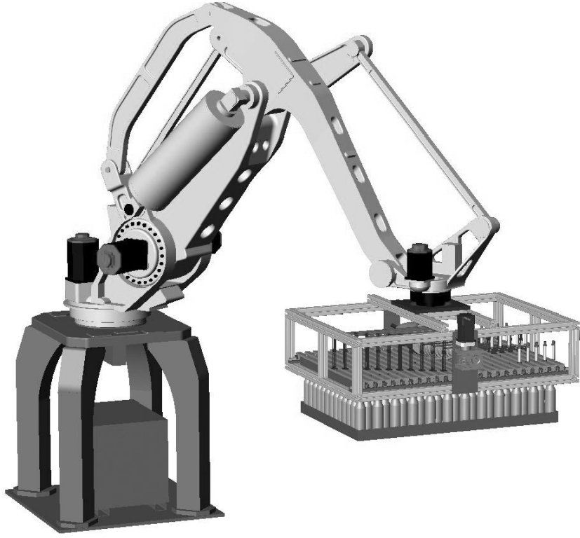
Şekil 3.2 - Payload 300kg 4 Eksen Palletizing Robotu + Universal Blower Tooling
